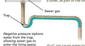
**Trap and vent** Nothing more than a connection to exterior air, a vent neutralizes air pressure within the drain lines.
