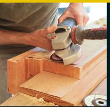
**Aggressive and cautious.** Use an angle grinder to pare down the end grain of the mitered returns, this time using an abrasive wheel that won't cause tearout.
