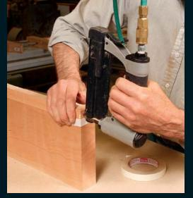
Frieze: wide, mitered returns. Glue the returns to the miters, using tape to hold each piece in alignment, then fasten the joint with a couple of pin nails.
