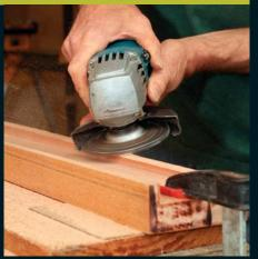
**Sneak up on the scribe.** After clamping the leg onto a worksurface, use an angle grinder equipped with a chainsaw carving blade. Check the fit, and adjust the scribe as needed.
