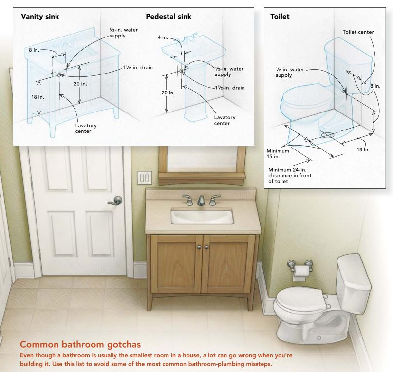
**Too-tight toilet.** While code requires only a 30-in. space for a toilet, 15 in. from a cabinet or adjacent wall can make you feel claustrophobic. Try for at least a 34-in. opening, and make sure there's space for the paper holder. Roughing in 13 in. instead of 12 in. from the back wall leaves room for the trim and the drywall.
